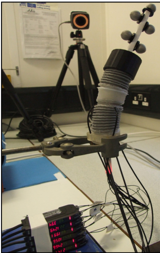
Figure 13: Calibration of the bending sensor
