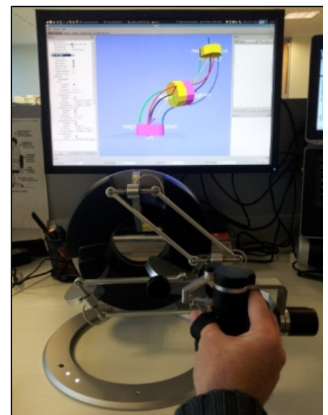
Figure 18: Omega 7 haptic device controlling simulated STIFF-FLOP arm
